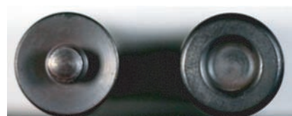
上搅拌头形貌 下搅拌头形貌 图 2 Concave-DFSW 搅拌头形貌 [19] Fig.2 Morphology of Concave-DFSW welding tools [19]
